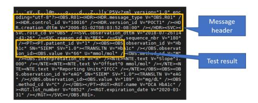
Figure 13 - Details of the POCT01 packet transmitting the HbA1c test results to the LIS.
