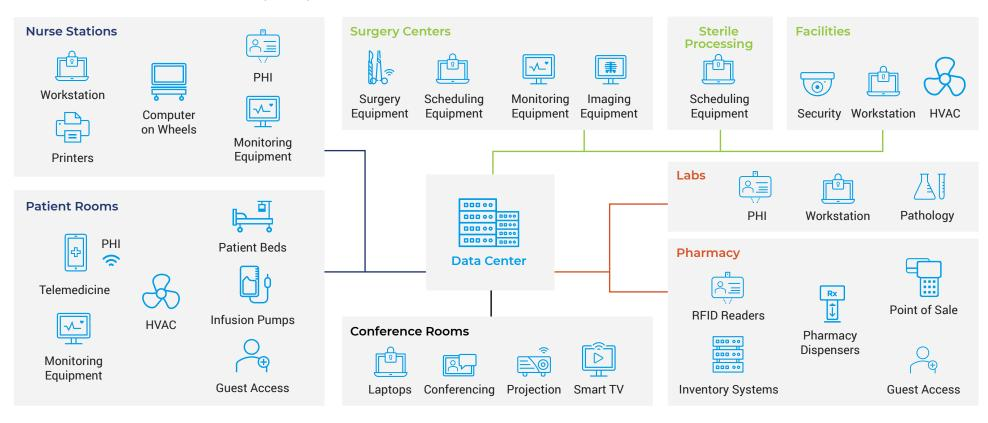
Figure 1 - Devices in a typical healthcare network.
