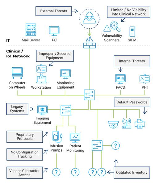
Figure 2 - Network diagram with potential threats.
