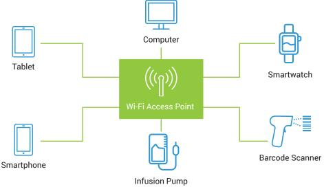
Figure 5 - Example of VLAN shared by smartphones, tablets, barcode scanners and healthcare devices.
