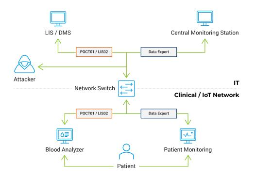
Figure 11 – Healthcare lab used for our attack demonstrations.
