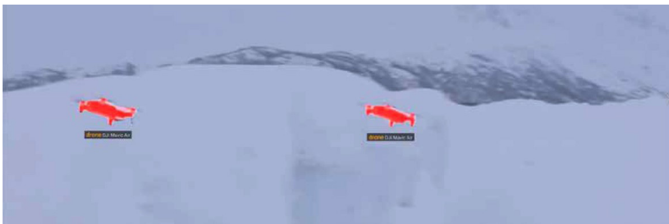
Figure 10: DroneShield's DroneOptID™ software detecting and classifying multiple white drones against a white arctic backdrop. Red overlay represents pixels identified as 'drone object' tracked by the software
