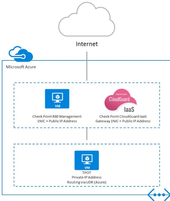
To demonstrate the value of using advanced threat prevention security for the cloud, we placed a Check Point CloudGuard IaaS Gateway in front of our TPOT and connected it to Check Point's Smart Center R80 management server.
