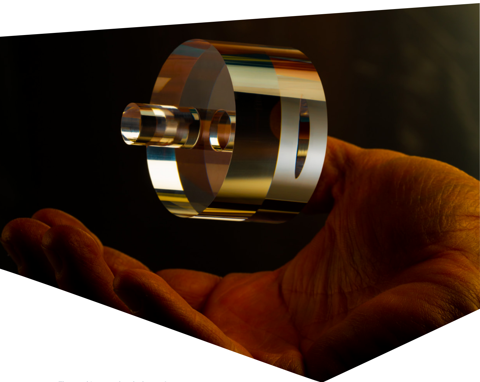
The sapphire crystal at the heart of one of the world's most precise clocks. Credit: QuantX Labs
