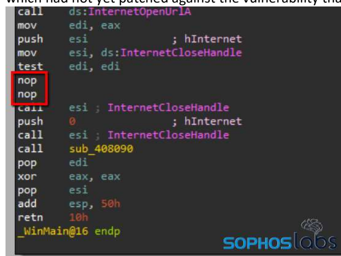
Figure 13: An example of a Wannacry executable with two "no-operation" commands instead of a kill switch subroutine
